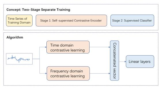
Figure 1: The framework of our two-stage separate training method. The different color of stage 1 and stage 2 means that they are trained separately and have no relation in principle.
